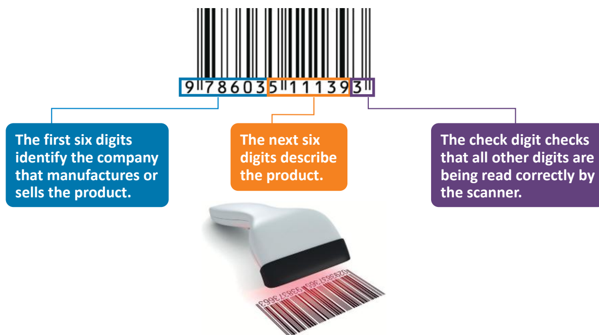
Figure 2.15: Example of barcode structure
