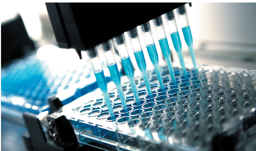
FIGURE 9–14 Robots can be used in research to fill pipettes with the correct amount of solution. ©iStock.com/David Gray
