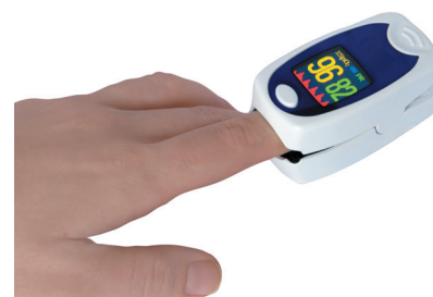
FIGURE 12–12 A pulse oximeter measures the percentage of oxygen in the blood. Many oximeters also measure the pulse rate per minute.
