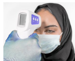
FIGURE 12-8 Non-contact infrared thermometers can measure the thermal energy radiating from the skin.
