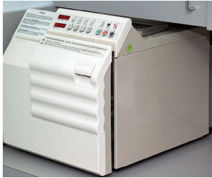
FIGURE 11-15 An autoclave uses steam under pressure or gas to sterilize items.
