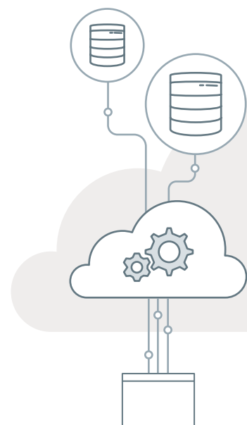
Figure 4.27: An application communicates with a cloud platform through a Web API
