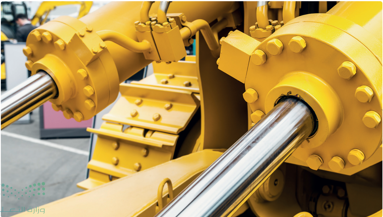
Figure 1.15: Hydraulic actuator (piston) system on heavy machinery
