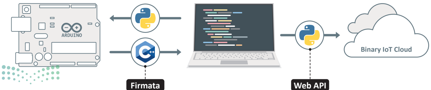
Figure 4.29: Arduino communicating with PC and Binary IoT Cloud
