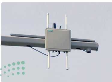
Figure 7.6: Roadside Unit (RSU)
