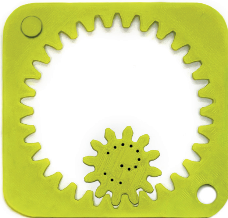
Printed Base of the spirograph.
