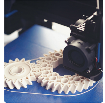
Figure 3.5: Gears produced by small black FDM printer
