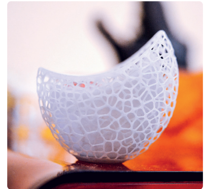
Figure 3.2: Object photopolymer printed on a 3D printer
