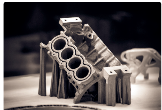
Figure 3.4: Object printed in laser sintering machine
