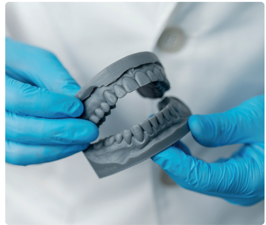
Figure 3.15: Upper and lower jaw printed on a 3D printer
