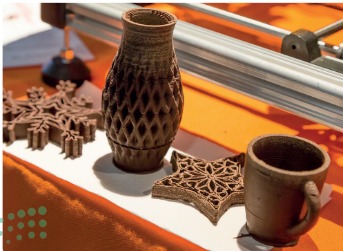
Figure 3.12: 3D Printing with ceramic material
